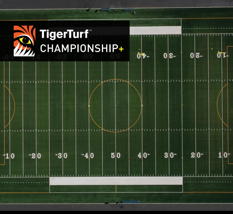
Combining durable XPS slit film and playable Diamond monofilament fibers with thatch at the base, players get a heavier, more consistent playing surface.
